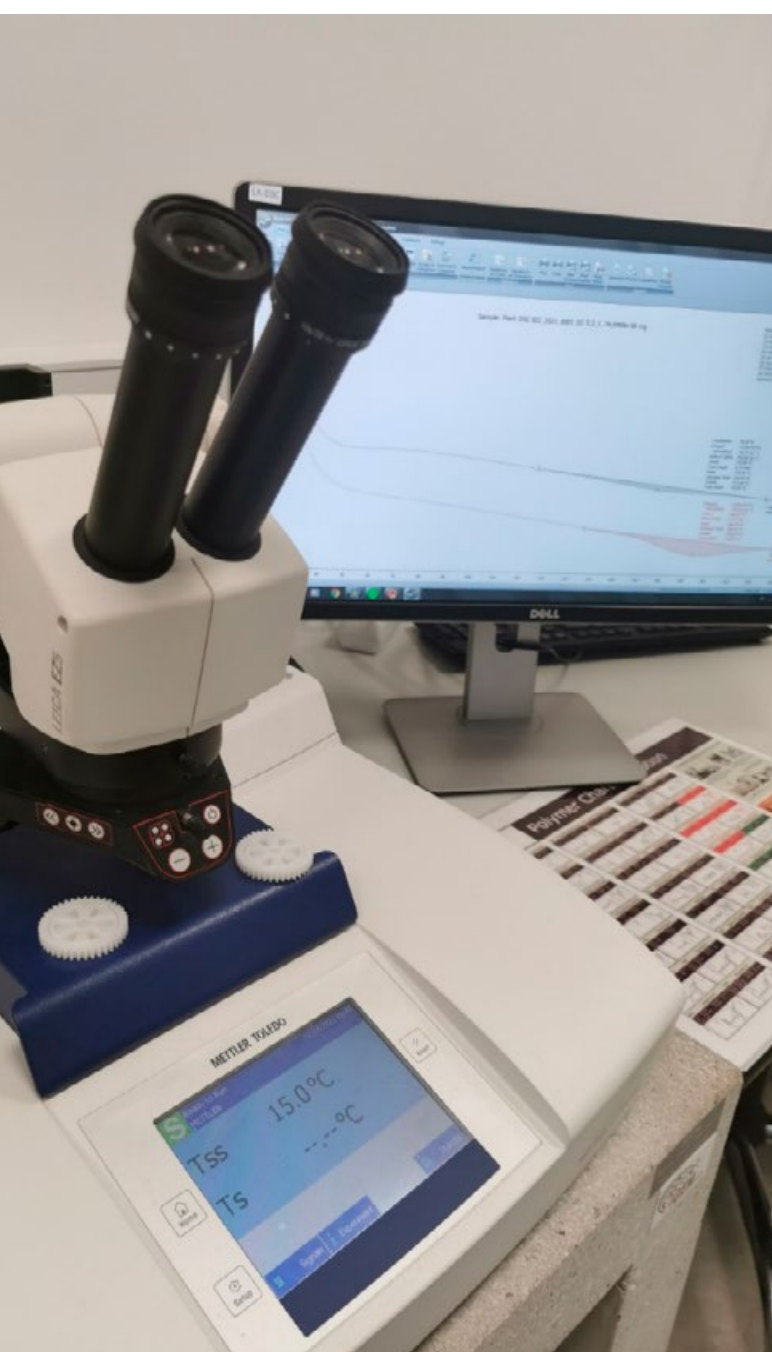
Flash DSC 1 (Mettler Toledo) s prototipi zobnikov
