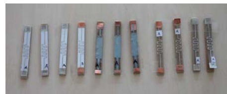
Figure 5: Samples made with IML technology
