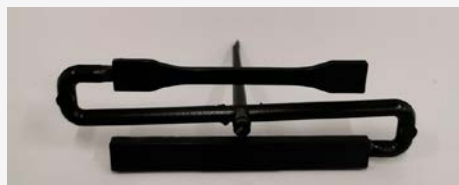
Figure 1: Injection moulded specimen sized according to ISO 527 (1BA) and ISO 178
