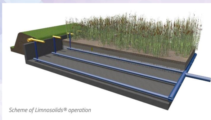
Sludge drying reed bed scheme (left) and live (right) (source: Limnos)
